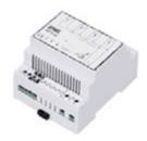
**1071/42 – Two-motor DIN module**: it can be installed on a DIN bar to manage two different motors. It receives phase and neutral from a magnetothermic switch, and manages every motor through three cables, controlling their interlocking. Dimensions (W  $\times$  H  $\times$  D) in mm: 72  $\times$  58  $\times$  90 - rated CUs: 3.5 - DIN modules: 4
